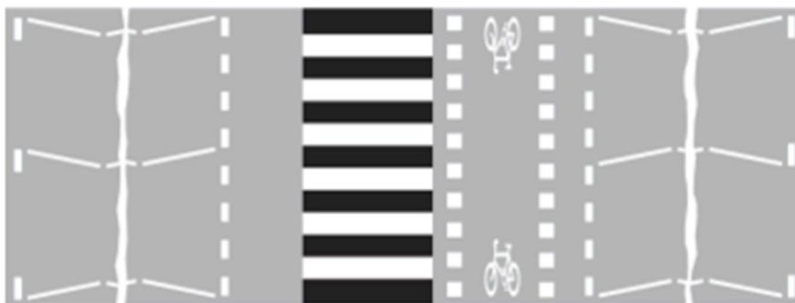
Figure 8-3: Parallel crossing to make provision for cyclists
